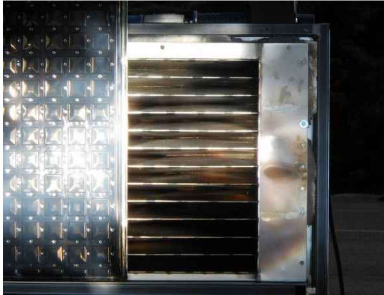
Figure 6: comparison between a conventional heat exchanger with wave length selectivity (left) to the new solar-air heat exchanger.
