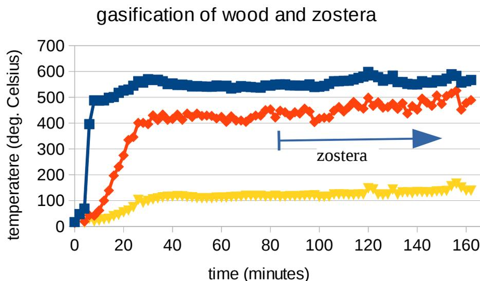
Figure 3: temperatures in the gasifier during the gasification of wood pellets (first 80 minutes) and *zosteramarina*.
