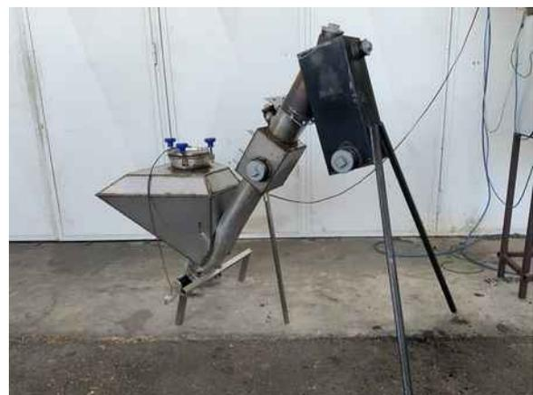
Figure 1: gasifier for solar carbon, thermal power 25 kW.
